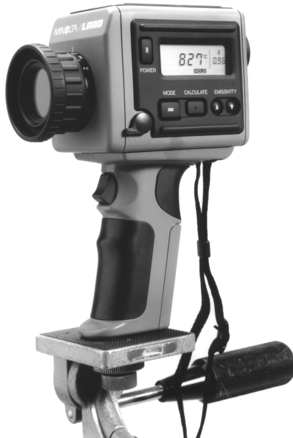
Figure 3.3. Photograph of an industrial spectral-band radiation thermometer.
