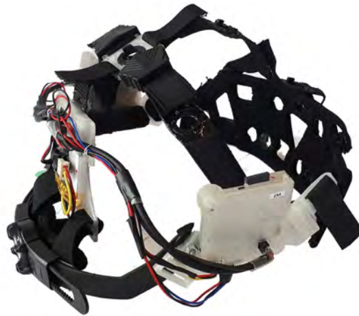
Von Lühmann's M3BA wearable device combines fNIRS with EEG imaging capability.
