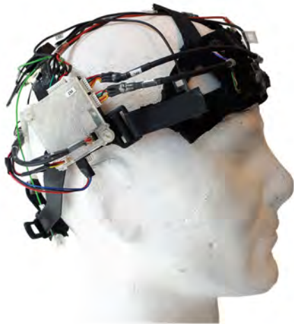
Von Lühmann's M3BA wearable device combines fNIRS with EEG imaging capability.
