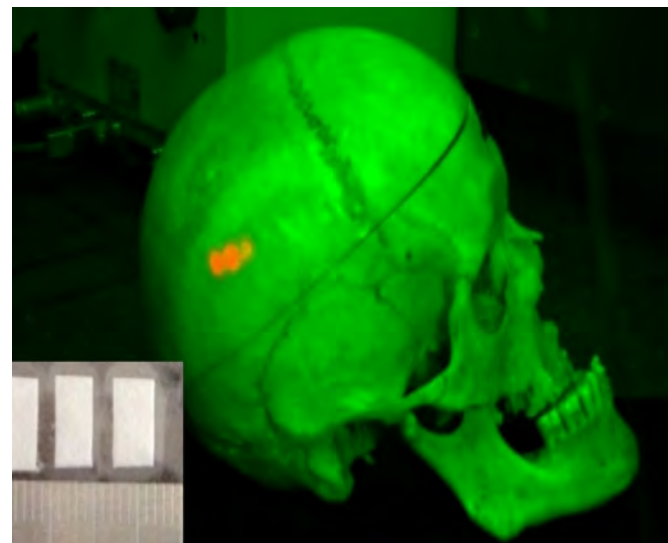
Through-skull imaging: Two-photon bioimaging using IR to IR up-conversion in rare-earth-element doped nanoparticles. Credit: Paras Prasad.
