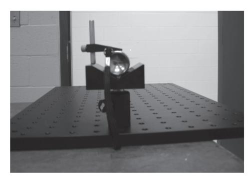
Figure 13 Beam Divergence Measurement Set-up
