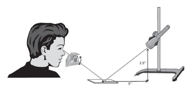
Figure 4 Polarizer with Analyzer Illustrated
