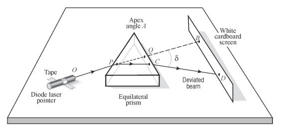
Figure 7Minimum Angle of Deviation Set-up
