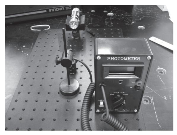
Figure 5 Filter Power Measurement Set-up
