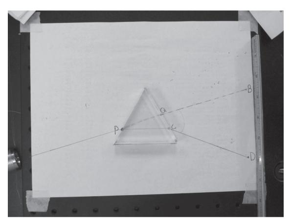
Figure 8 Minimum Angle of Deviation Set-up
