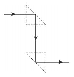
Figure 9 Total Internal Reflection Set-up
