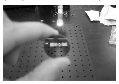
Figure 3 Polarization by Reflection Set-up
