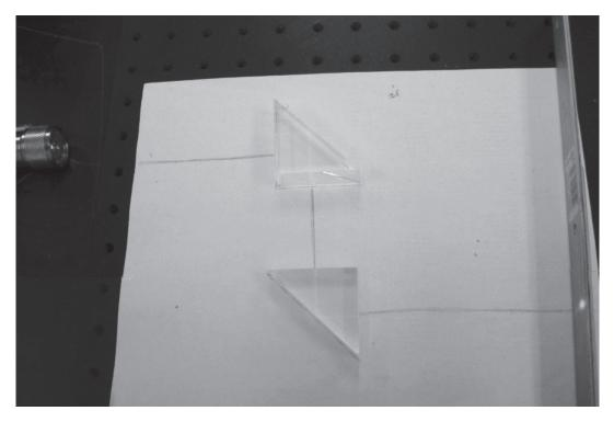
Figure 10 Total Internal Reflection Set-up
