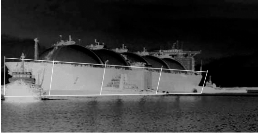
Figure 14 Example of infrared system used for harbor security. White lines mark the virtual perimeter.
