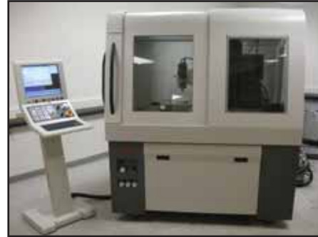
Micro Milling machine for generating wafer-based lens arrays (>2000 cavities) to the highest accuracies.
