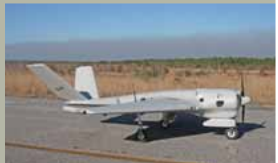
DRS Sentry HP Unmanned Aerial System
